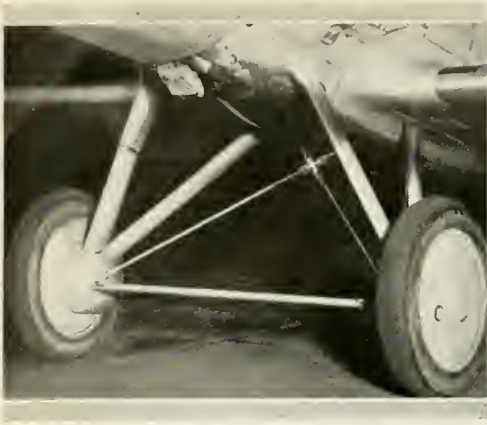
Fig. 5. Brake-equipped spreader type landing gear
